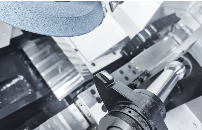
测量模板磨削 Gauge Template Grinding
