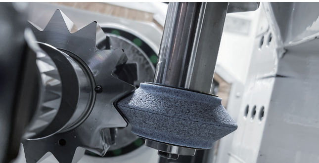
三角花键磨削 Triangular Spline Grinding
